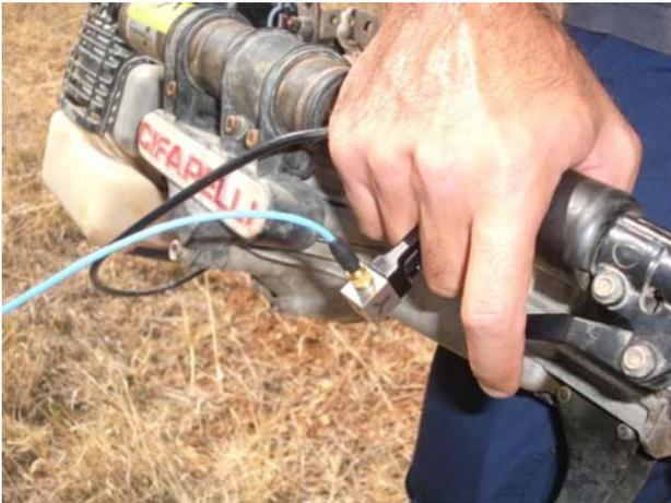
Figure 4 Triaxial accelerometer and its adapter used in the tests
