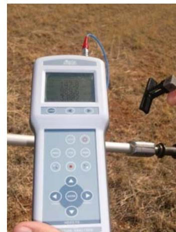
Figure 3 HD2070 vibrometer used in the tests
