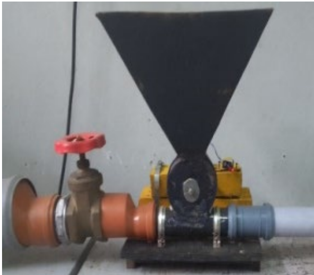
(c) air flow control and feeding system
