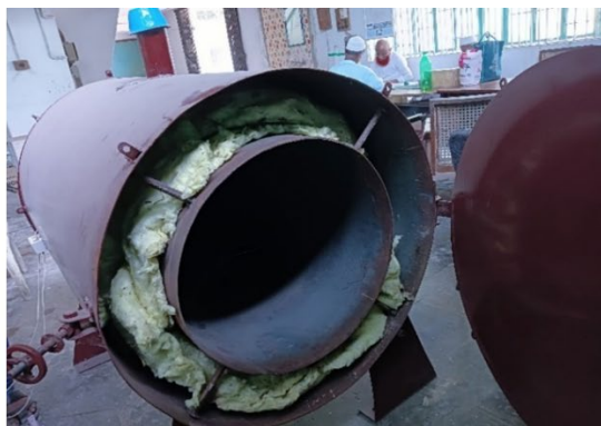
(c) glass wool between inner and outer cylinder
