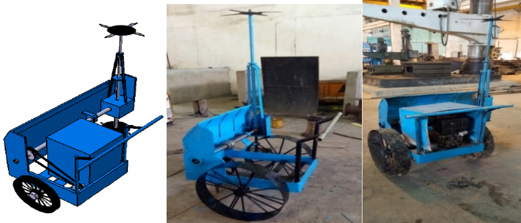
Figure 12 Machine model and construction of machine in the shop
