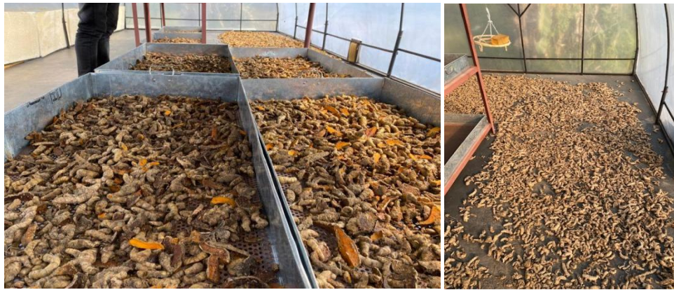
Figure 18 View of the GHD under loaded condition of turmeric
