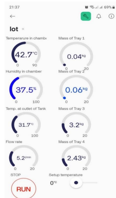
Figure 5 Blynk interfaces for displaying dryer parameters 2.2.4 Arduino control system for heating management We developed the Arduino program. It allows users to select operating modes via a keypad (0-4)
