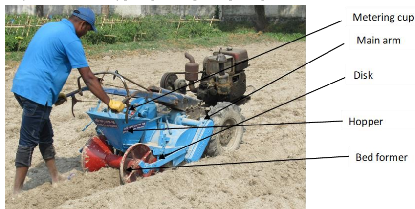
Figure 7 The improved potato planter and its important functional parts
