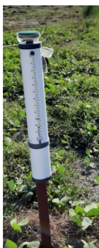
Figure 1 (left) Atmometer (right) Estimated evapotranspiration of sweetpotato in San Felipe, Zambales (From planting to harvesting)
