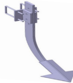
Figure 5 Shank in an attachment position with the blade 2.2.7 Design of wheel
