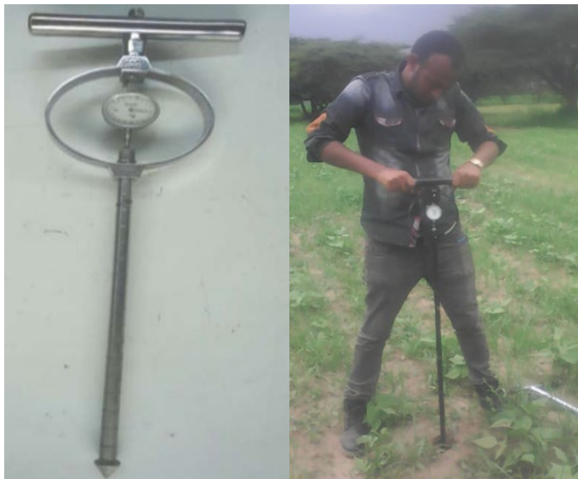
Figure 9 Penetrometer for measurement of cone index
