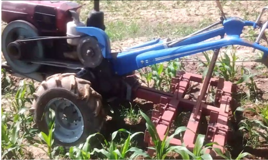
Figure 10 Pictorial view of the 2WT drawn cultivator
