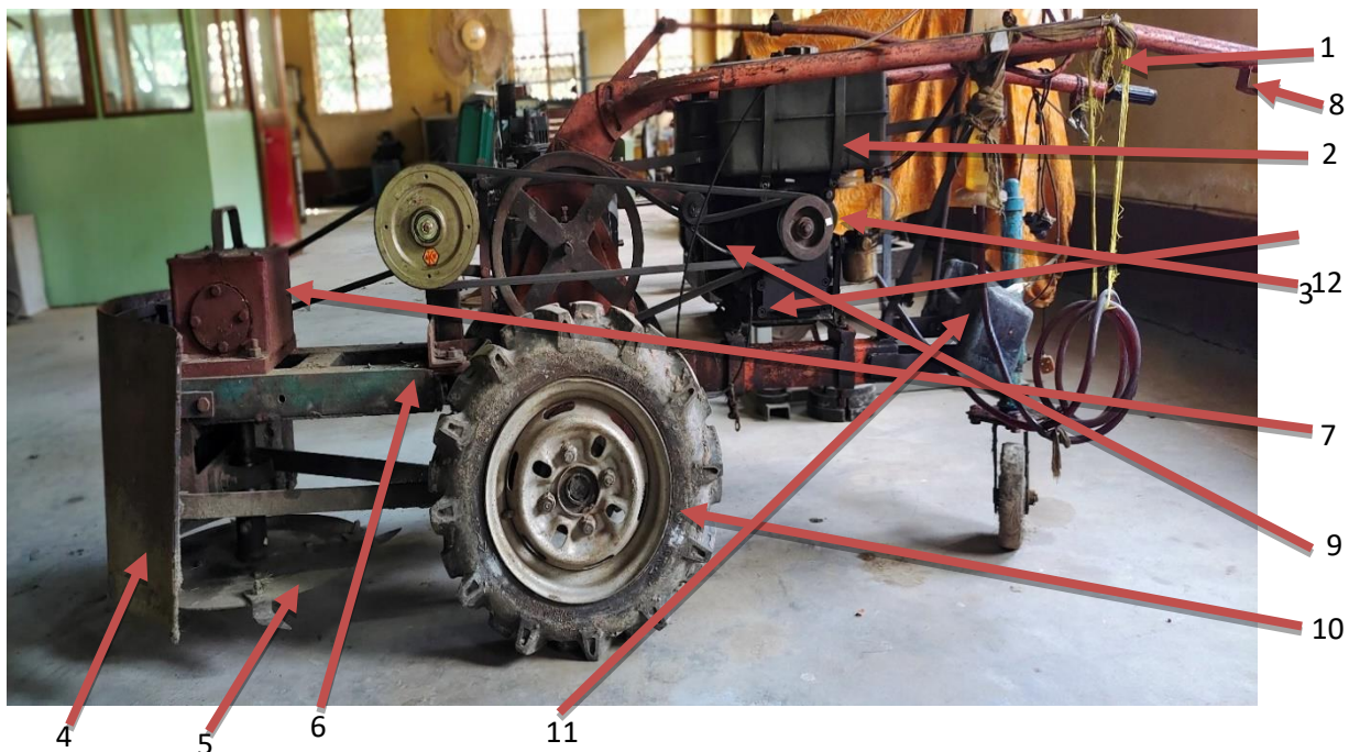
1. Drive gear lever, 2. 6.5 Hp engine, 3. Frame, 4. Guard Plate 5. Rotary cutting disc 6. Main frame, 7. Gear box, 8. Accelerator, 9. Belt Drive 10. Wheel, 11. Counter weight, 12. Pulley
