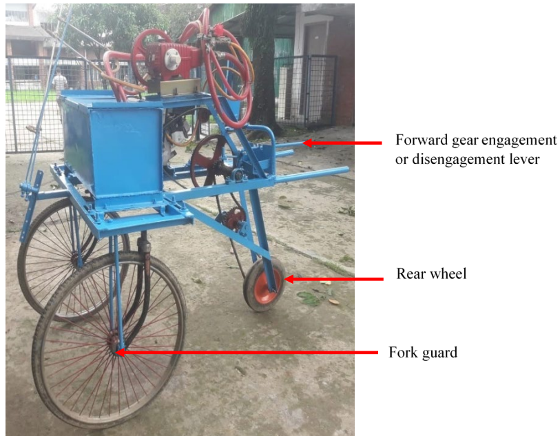
Figure 3 The major components and operational aspects improved in the boom sprayer (Developed during 2022-2023)
