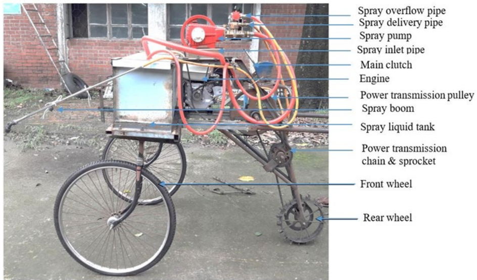
Figure 2 The primary components and operational elements of the boom sprayer (Developed during 2021-2022)
