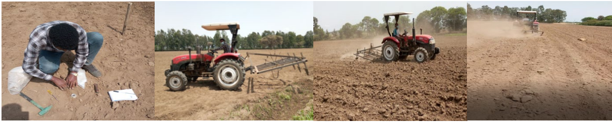
Figure 7 Field test of tie ridger machine
