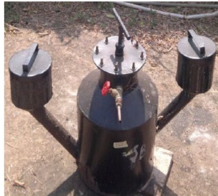
Figure 1 Constructed 48 liters fixed dome biodigester
