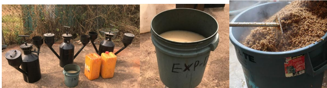
(a)fixed dome biodigesters, (b) cassava wastewater(CWW) and, (c) spent grain (SG)
