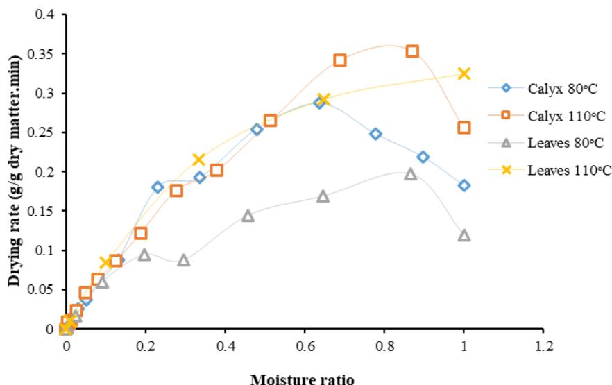
Figure 3 Drying rates of infrared dried Roselle calyces and leaves
