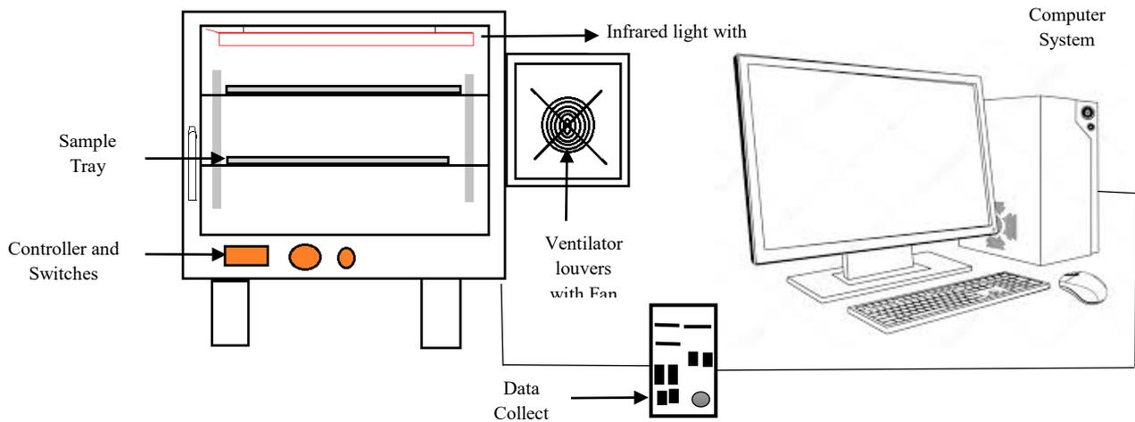
Figure 1 Schematic diagram of a laboratory infrared dryer
