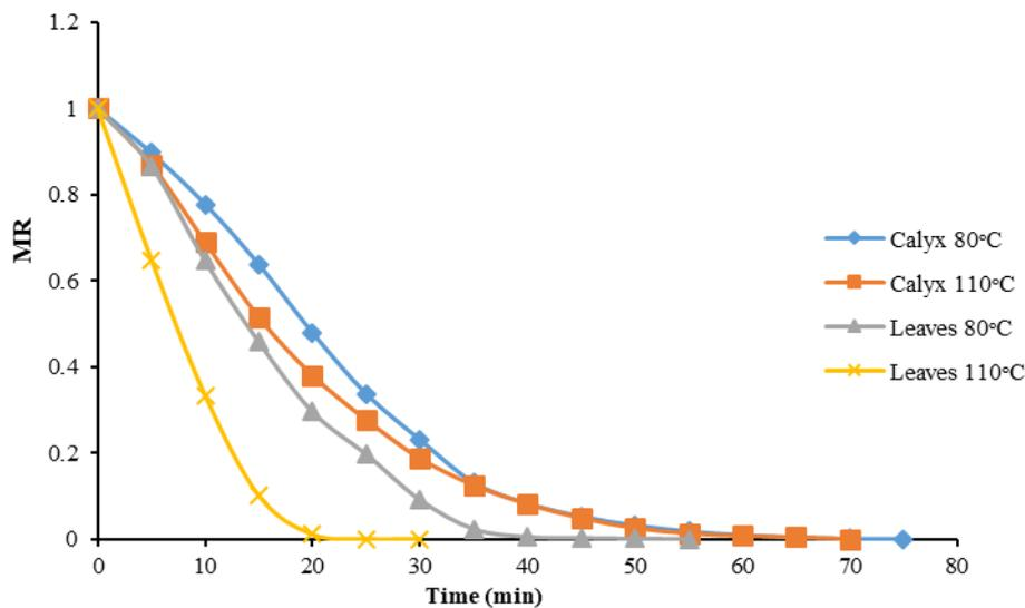
Figure 2 Moisture ratio (MR) of infrared dried Roselle calyces and leaves
