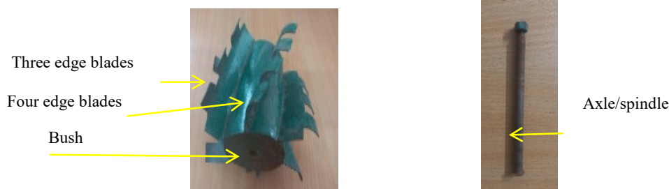
Figure 8 Photographic view of the rotor of the weeder with serrated blades, axle or spindle, and bush
