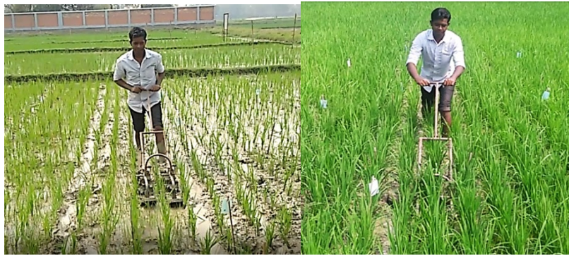
Figure 14 Field performance of the double-row weeder (Final version)
