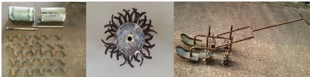
Figure 1 Photographic view of the double-row weeder and its parts (First version)
