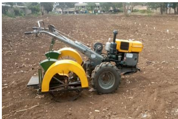
Figure 1 Developed power tiller drawn sunflower planter
