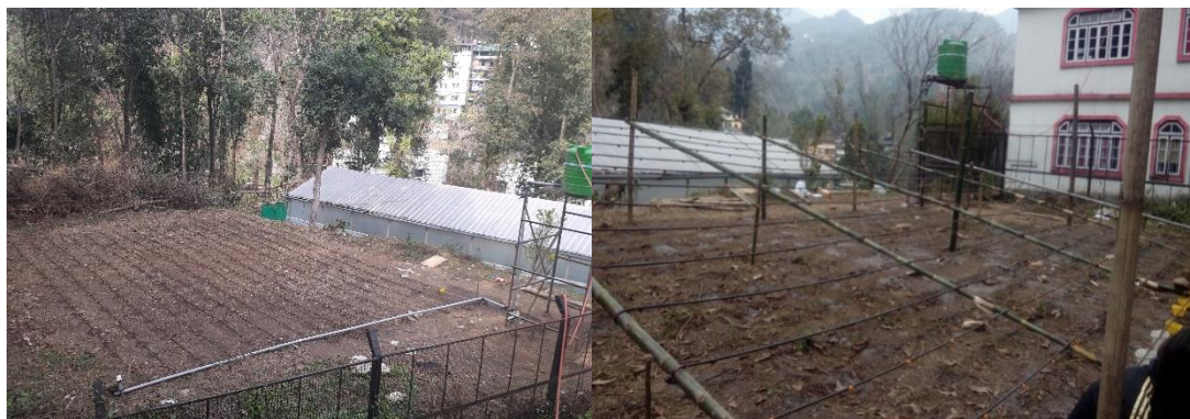
Figure 3 Experimental field view of gravity drip system at 0% slope and 3.0 m tank height and at 10% slope and 3 m tank height
