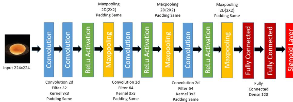
Figure 4 Architecture of the proposed CNN model
