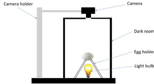
Figure 2 The system for taking the raw salted egg images
