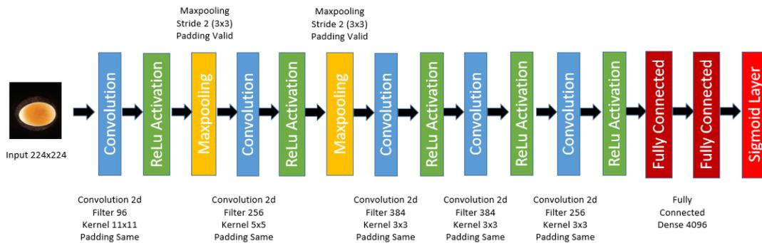
Figure 5 Architecture of AlexNet
