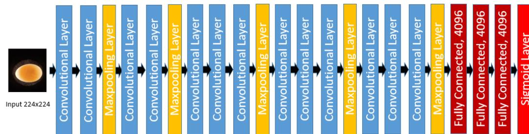
Figure 6 Architecture of VGG-16
