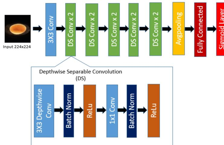
Figure 8 Architecture of MobileNet
