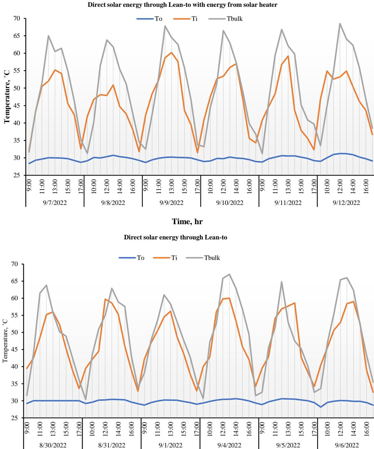
Figure 7 Illustrates the daily fluctuations in bulk and ambient temperatures, both inside and outside the solar collector, over the course of the experiment for the two distinct systems
