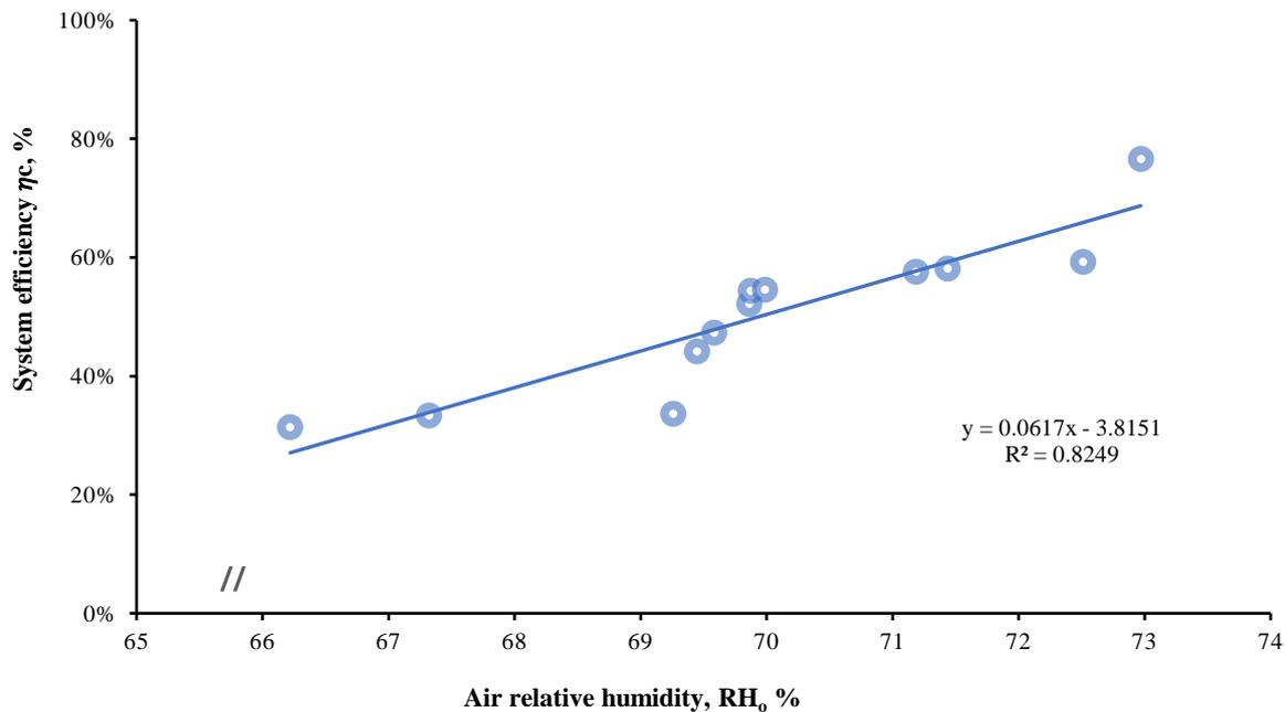
Figure 10 Depicts the direct correlation between system efficiency and incident solar radiation, ambient temperature, and relative humidity
