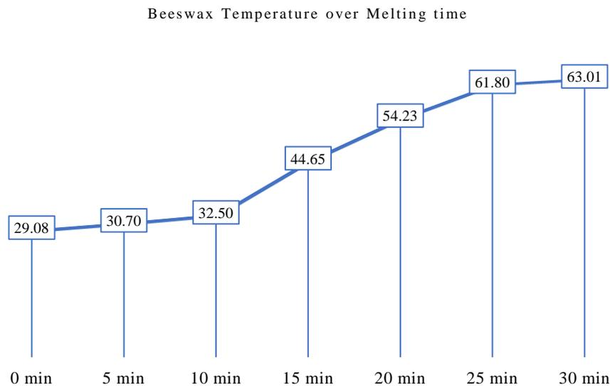
Figure 4 Beeswax temperature during melting using a water bath
