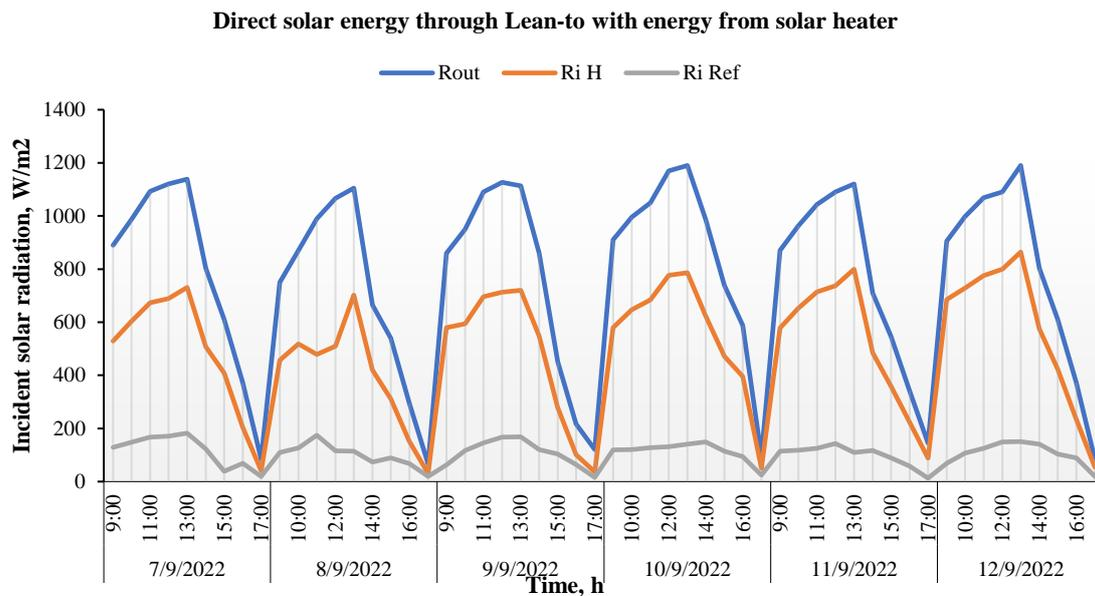
Figure 5 Depicts the daily fluctuations in incoming solar radiation, both within and outside the collector, along with the reflected radiation from the vertical-back wall during the experimental period for the two systems
