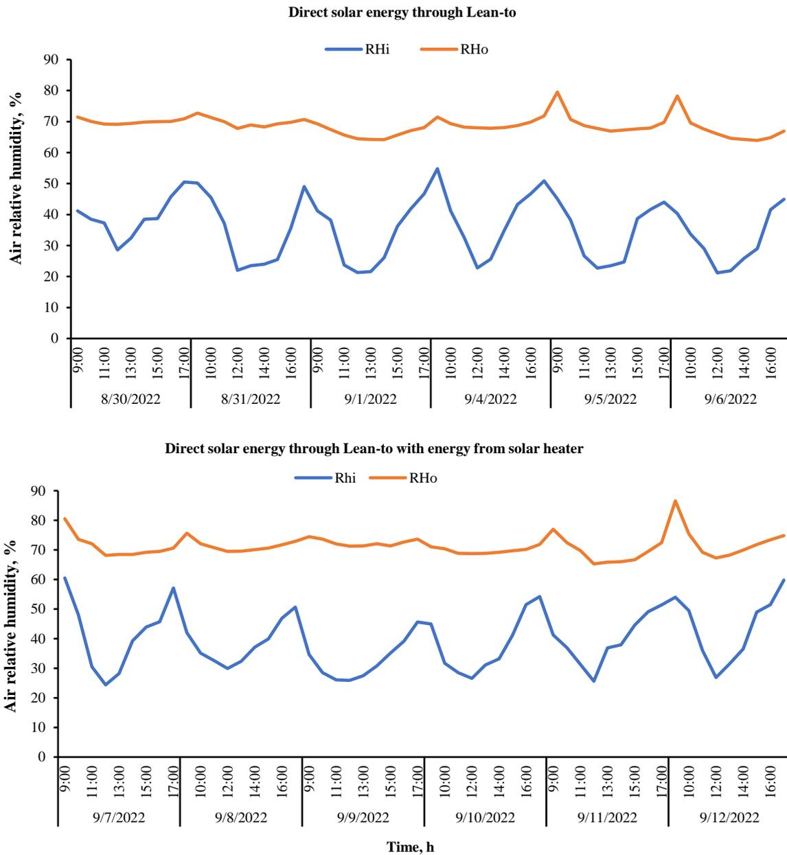
Figure 9 The daily variations in relative humidity levels both inside and outside the solar collector were monitored throughout the experimental period for the two systems
