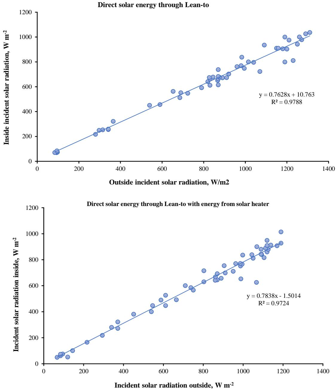
Figure 6 Illustrates the correlation between the incident solar radiation within the solar collector and the incident solar radiation outside for both systems
