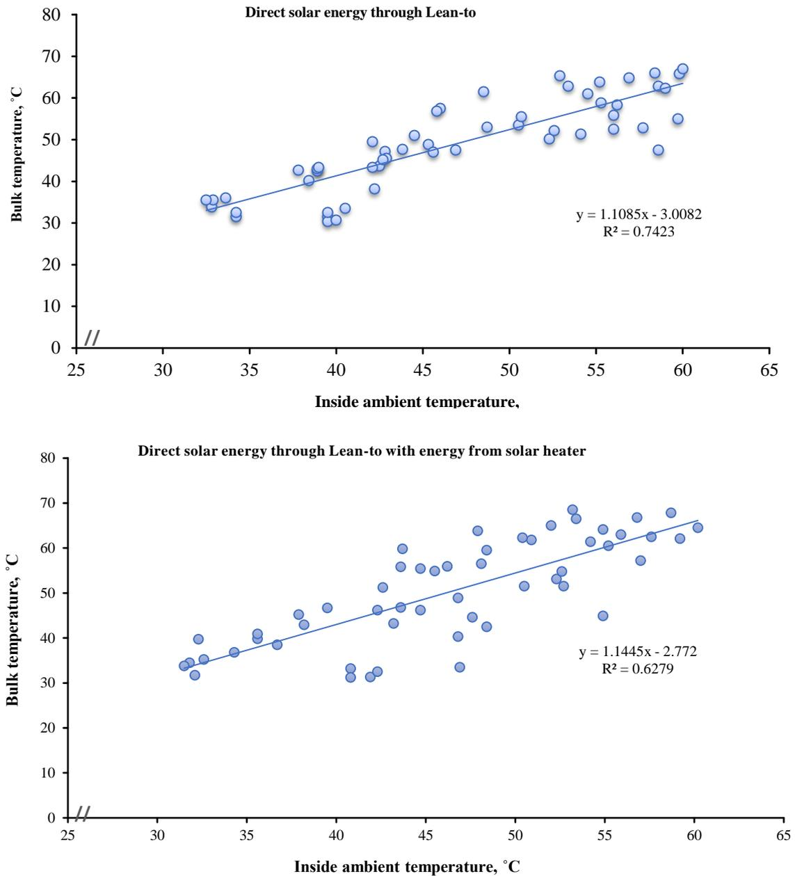
Figure 8 Displays the correlation between the bulk temperature of beeswax and the indoor ambient temperature within the lean-to solar collector for both of the investigated systems
