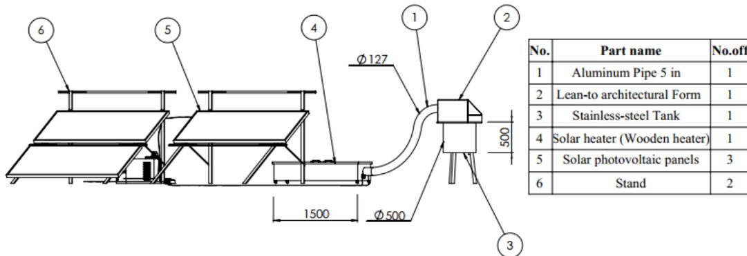
Figure 1 2D of the solar wax melter
