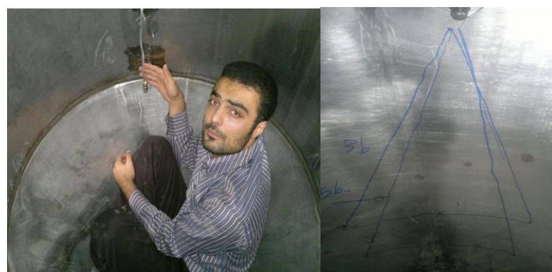
Figure 15 The effect of using air pressure nozzle to broom particles on the cone wall
