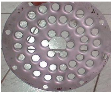
Figure 2 The circular distributor plate of the spray dryer
