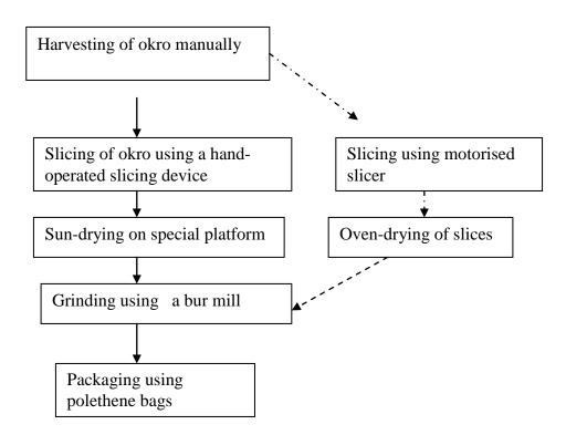
Fig. 1. Recommended flow chart for okro processing
