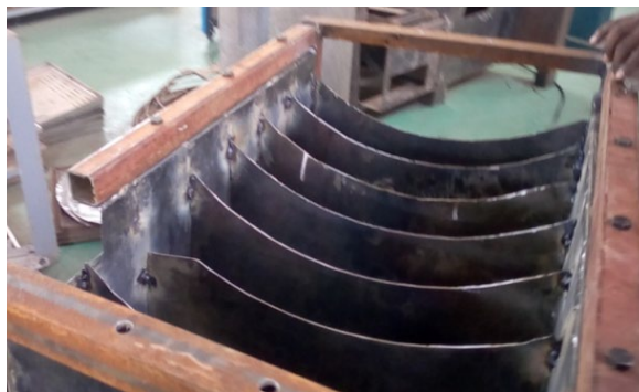
Figure 6 Sample ( tef , straw and chaff mixture) collectors box 1-7
