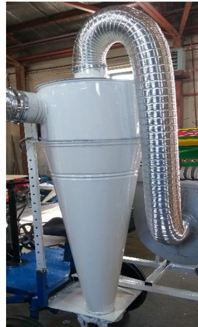
Figure 9 fabricated cyclone mounted on the machine chassis
