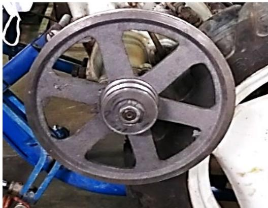
(A) drive-centrifugal fan pulley
