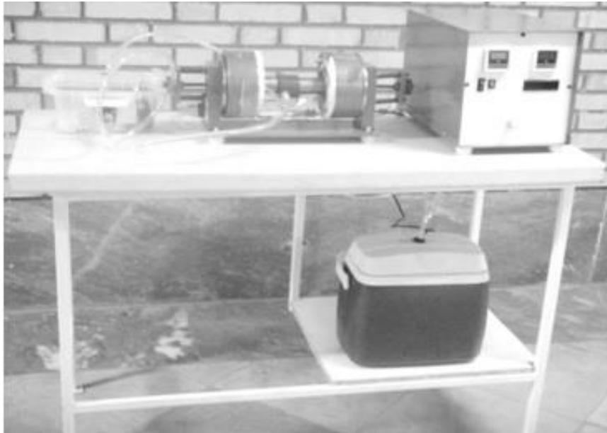
Figure 1 Magnetic water treatment devices
