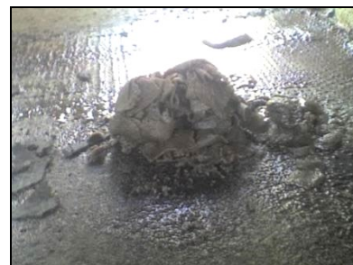
Figure 3 Paste discharged from expeller when expressing oil from seed kernel only
