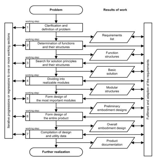
Figure 1. General VDI-procedure of systematic development and design (VDI 2221, 1993).
