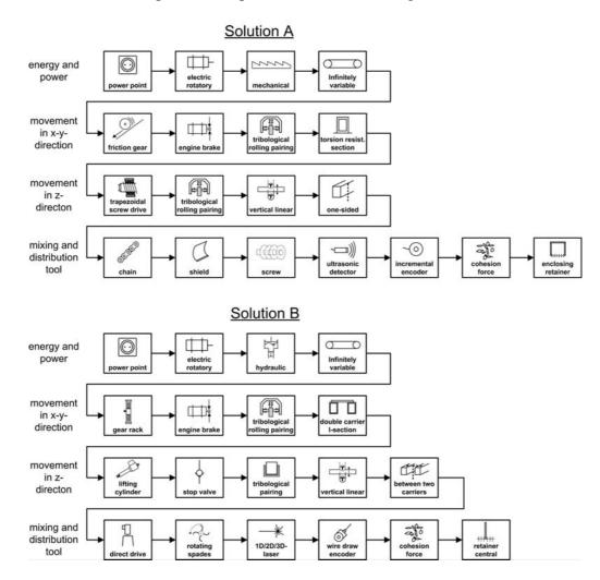
Figure 3. Preferred implementation solutions for each sub-function of the two solutions for the robot.
