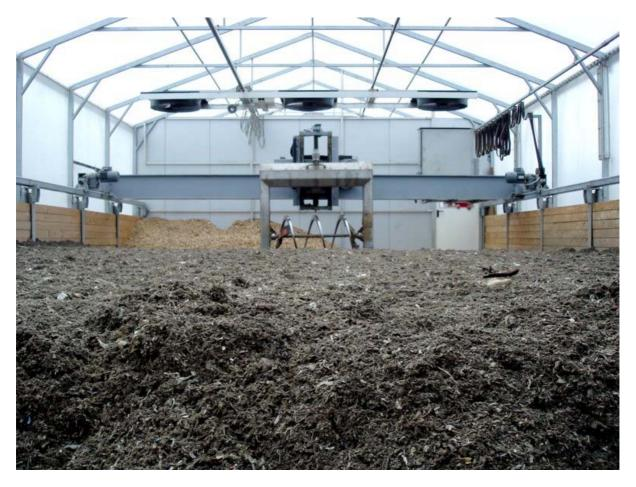
Figure 5. Prototype of the "Biomass-Manager" during an experiment in a solar greenhouse type dryer. The robot is processing a biowaste-paper blend.
