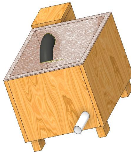
Figure 7 The 3D view of the cooling chamber
