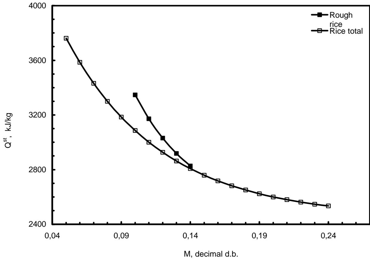
Fig. 5. Sorption isosteric heats of rough rice and rice total isotherms
