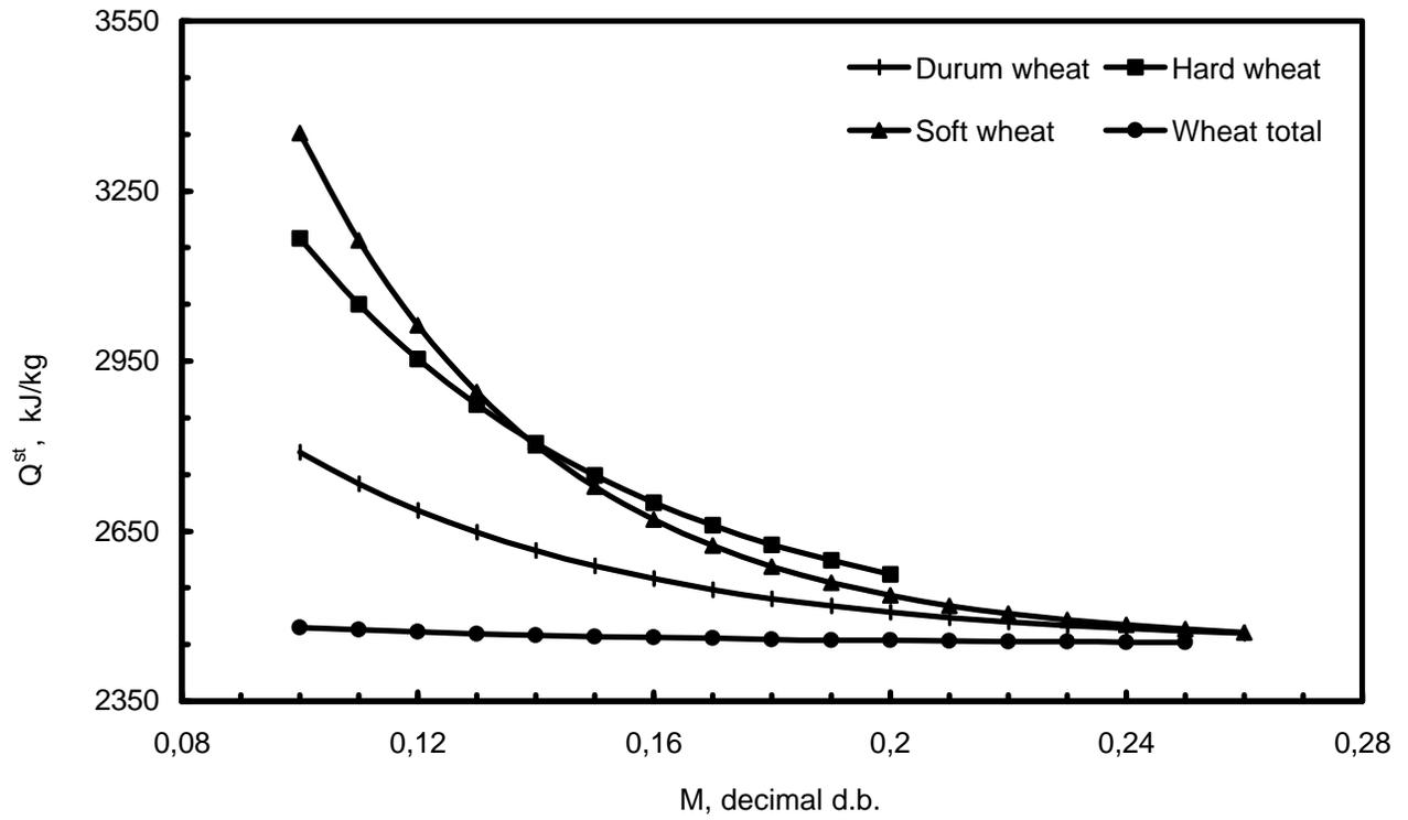
Fig. 3. Sorption isosteric heats for several wheat cultivars and wheat total isotherms
