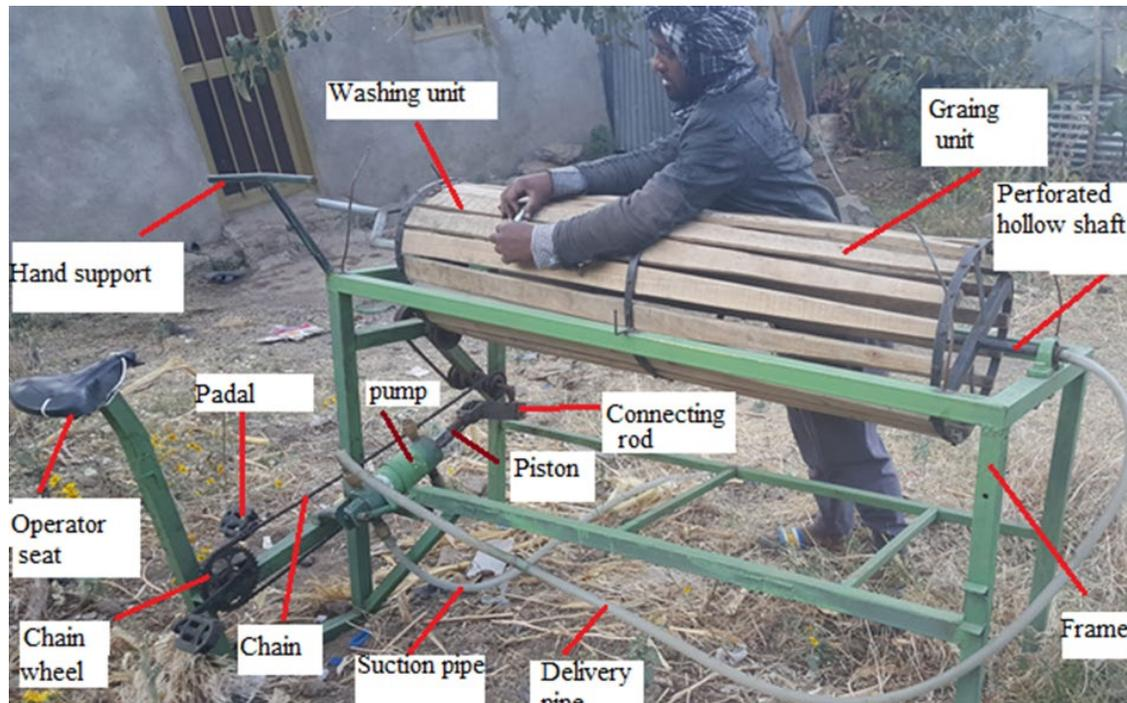
Figure 1 Manufactured carrot washing and grading machine
