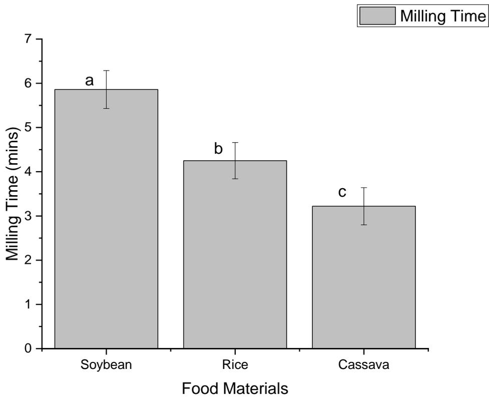
Figure 8 Milling time of soybean, rice and cassava flake. Graph bars with different superscripts (a, b and c) indicate significant differences among the food materials with the milling time ( $p < 0.05$ )
