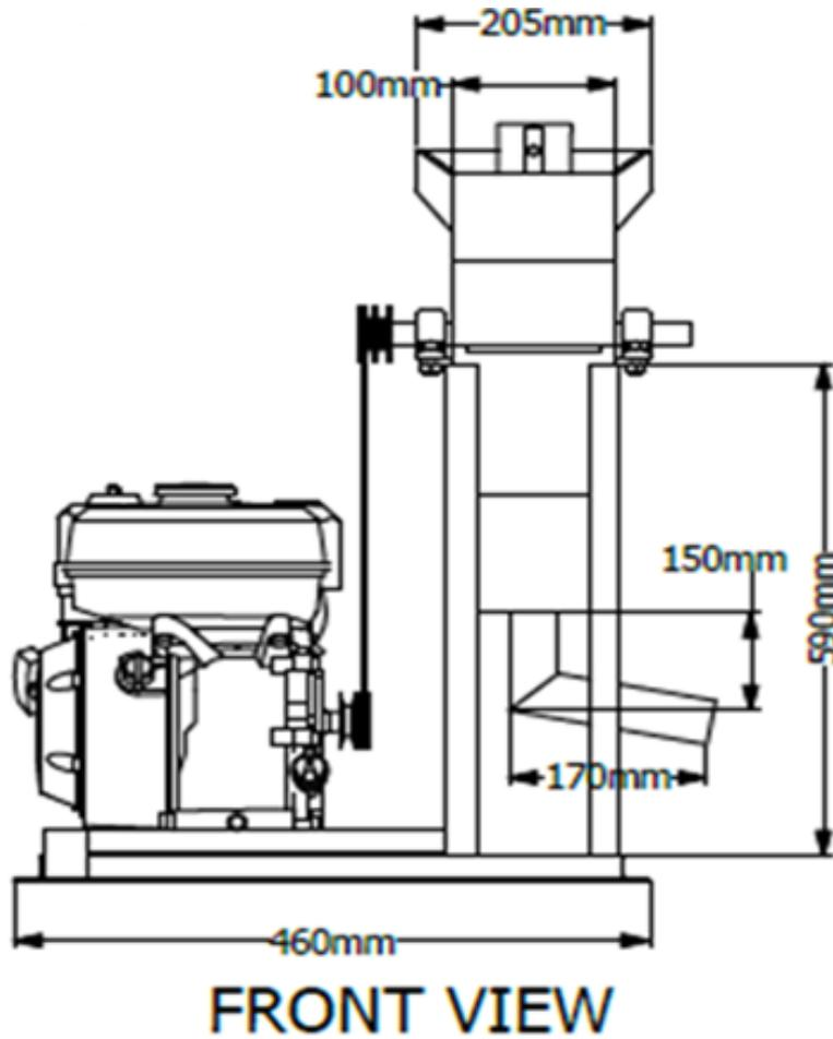
Figure 4 Front view of the gasoline food grade magnetic hammer mill
