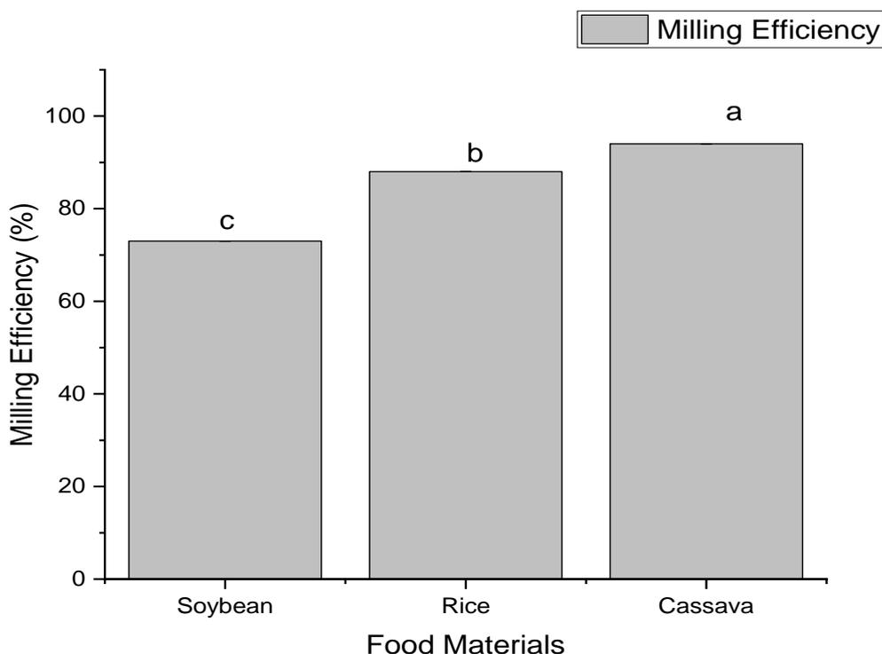
Figure 6 Milling efficiency of soybean, rice, and cassava flakes. Graph bars with different superscripts (a, b, and c) indicate significant differences among the food materials with the milling efficiency ( $p < 0.05$ )
