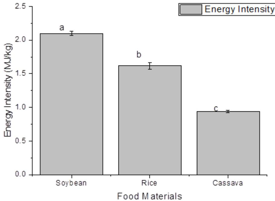
Figure 10 Energy intensity of soybean, rice and cassava flake. Graph bars with different superscript (a, b and c) indicate significant differences among the food materials with the energy intensity ( $p < 0.05$ )
