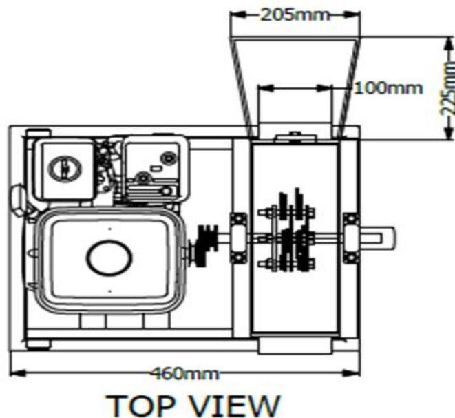
Figure 2 Top view of the gasoline food grade magnetic hammer mill
