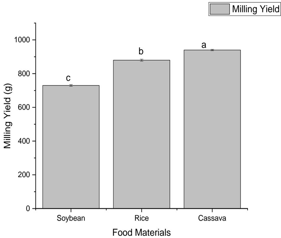
Figure 7 Milling yield of soybean, rice and cassava flakes. Graph bars with different superscripts (a, b and c) indicate significant differences among the food materials with the milling yield ( $p < 0.05$ )
