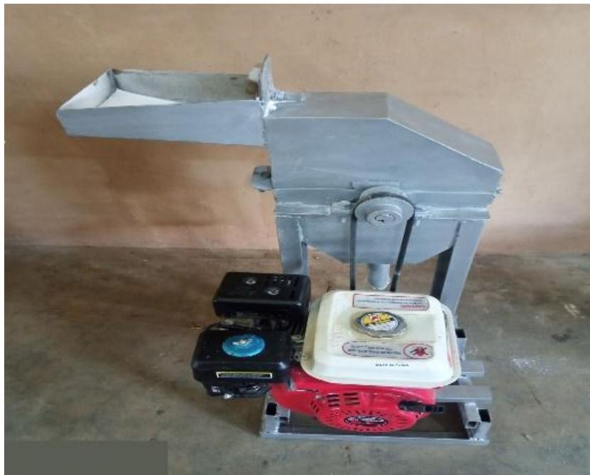
Plate 1 Pictorial view of the developed gasoline food-grade magnetic hammer mill
