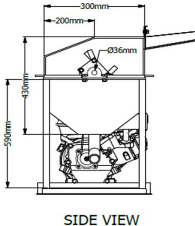
Figure 5 Side view of the gasoline food grade magnetic hammer mill
