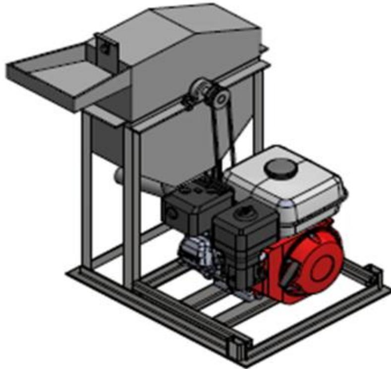
Figure 3 Isometric view of the gasoline food grade magnetic hammer mill
