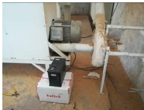
Figure 3 Three-phase electromotor and inverter installed on the peeling machine
