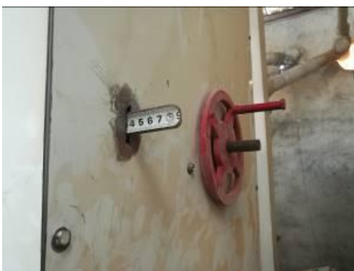
Figure 2 Blade connected to the machine inlet valve and its adjusting pulley
