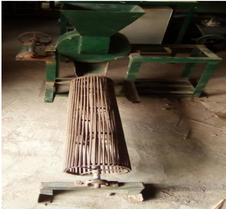
(b) Plate 1 Pictorial view of the developed palm kernel cracker
