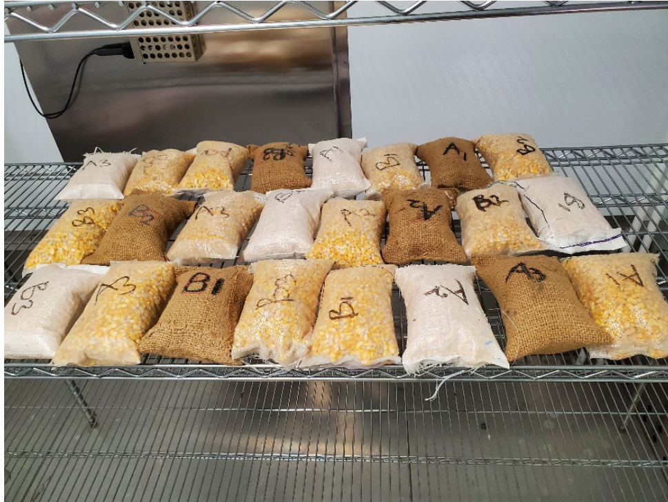
Figure 2 Experimental set up showing corn in mini-bags made with jute, polypropylene, and polyethylene (From left to right first row: PP-O, PE, jute, PP-C, PE, PP-O, jute, and PP-C).
