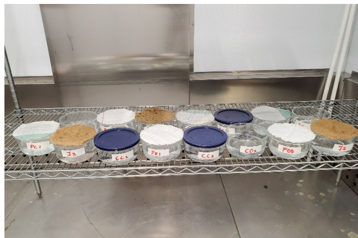
Figure 1 Experimental set up with glass containers in a random array with open dishes and those covered with plastic lids and bag materials (Left to right first row: PP-C, jute, covered dish, PP-O, covered dish, open dish, PP-O, and jute)
