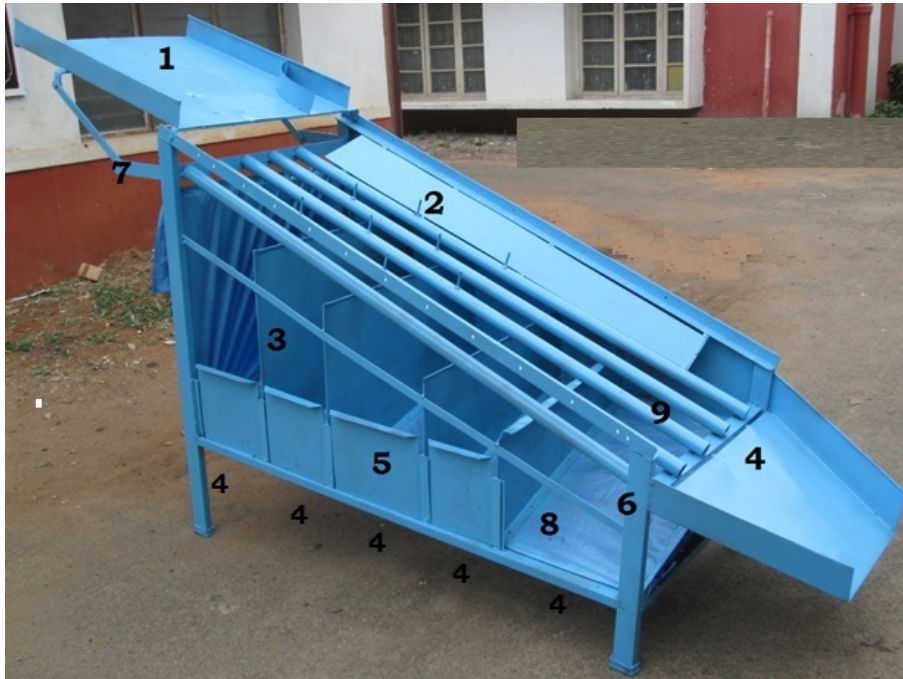
Figure 2 A gravity fed divergent type cocoa pod grader
