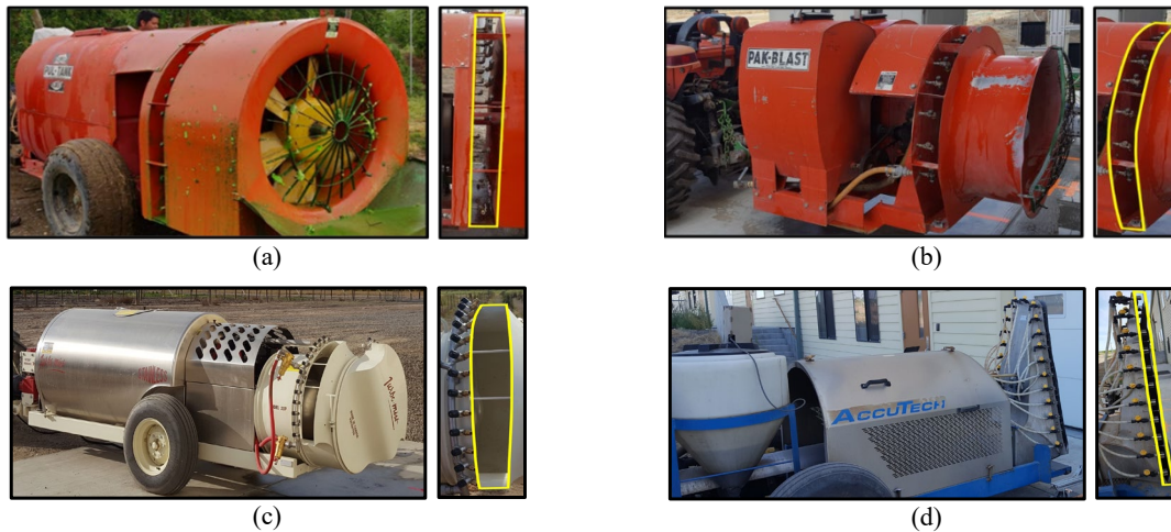
Figure 1 Commercial airblast sprayers (a) S1, (b) S2, (c) S3, and (d) S4 evaluated in this study. Solid yellow outlines to the right of each sprayer show pertinent air outlets
