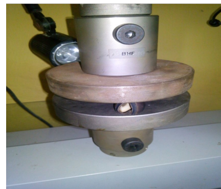
Figure 2 Cracking of the seed by compression using a UTM Oduma et al. (2016) in a similar study for African oil bean seed used 2.5mm min -1 . The behavior of the seed to
