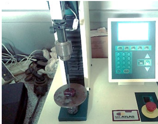
Figure 2 Location on the fruit where firmness were measured by penetration probe
