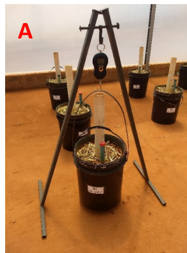
Figure 1 Experiment overview, showing the buckets with the access tubes and tensiometers installed.
