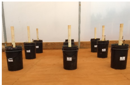
Figure 1 Experiment overview, showing the buckets with the access tubes and tensiometers installed.
