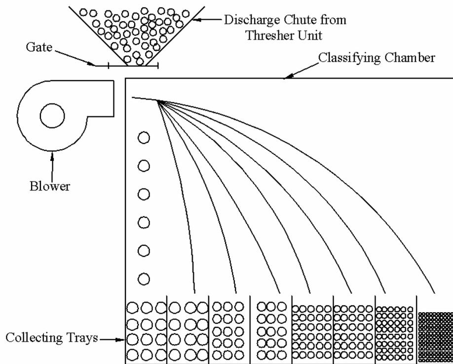
Fig. 5: Sketch of the Experimental Set up and Material Flow in the Classifier
