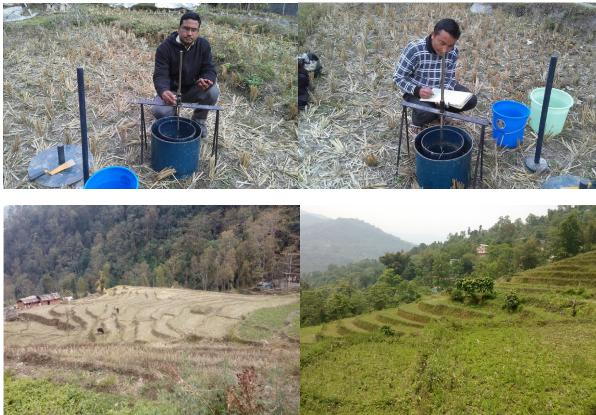
Figure 2 Infiltrometer test and paddy terraces at varying elevation
