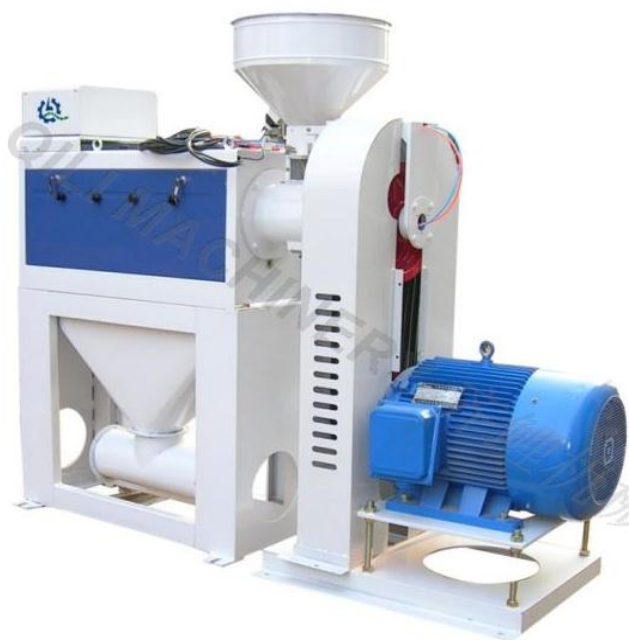
Figure 1 The machine (Satake KB40 type), used for husking paddy
