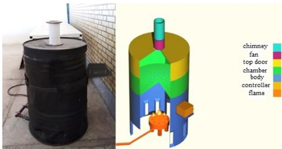
Figure 1 Schematic and real images of fabricated biochar production apparatus.
