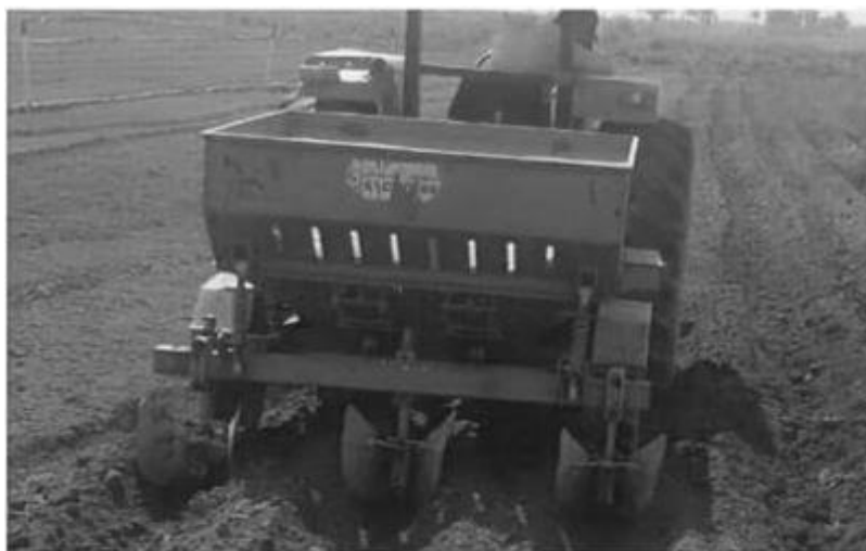
Figure 1 The machine (type Adwhit) used for potato planting
