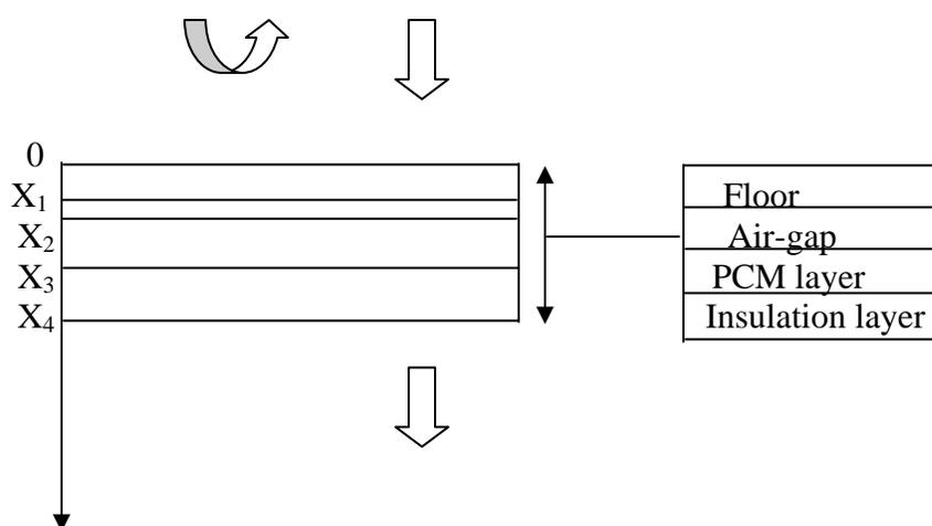
Figure 1(d). Schematic view of PCM floor.
