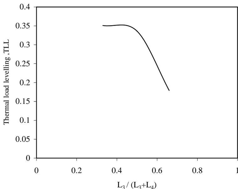
Figure 6. The variation of thermal load levelling (TLL) with different thickness of PCM and insulation, keeping the total floor thickness constant.
