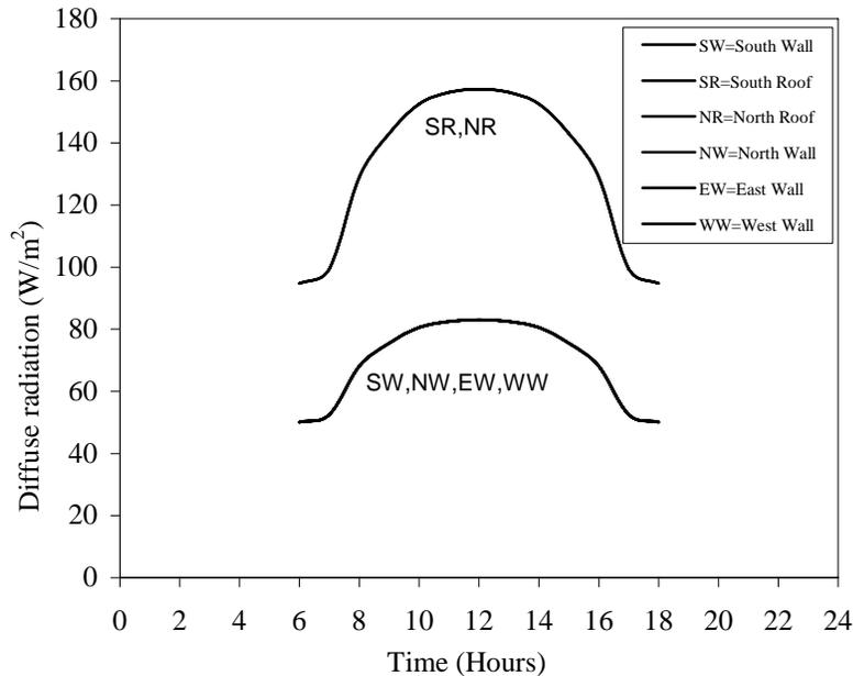
Figure 2. Hourly variation of diffuse radiation on different walls and roofs of greenhouse for a typical winter day in New Delhi.
