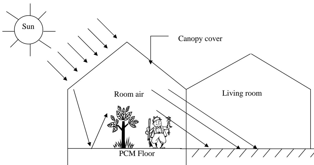
Figure 1(c). Greenhouse-cum-Solarium with basement having air-PCM.
