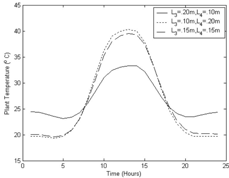
Figure 5(a). Hourly variation of plant temperature at different surfaces of floor varying thickness of PCM and insulation, keeping total thickness of the floor constant.
