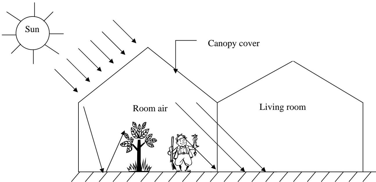
Figure 1(a). Schematic view of Greenhouse-cum-Solarium.
