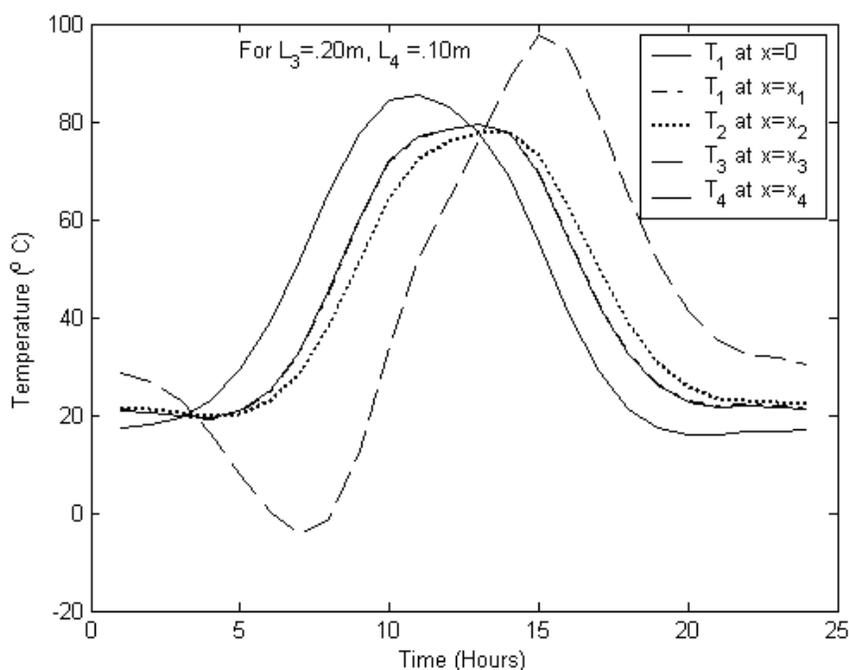
Figure 4(a). Hourly variation of temperature distribution at different surfaces of floor varying thickness of PCM and insulation, keeping total thickness of the floor constant  $L_3= 0.20$  m and  $L_4= 0.10$  m.
