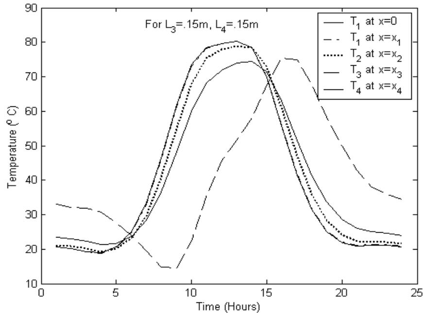
Figure 4(b). Hourly variation of temperature distribution at different surfaces of floor varying thickness of PCM and insulation, keeping total thickness of the floor constant  $L_3 = 0.15$  m and  $L_4 = 0.15$  m.
