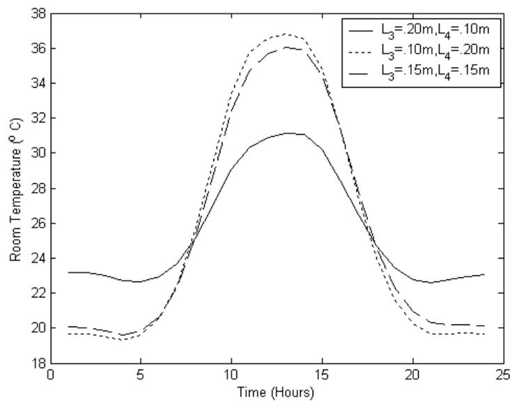
Figure 5(b). Hourly variation of room temperature at different surfaces of floor varying thickness of PCM and insulation, keeping total thickness of the floor constant.
