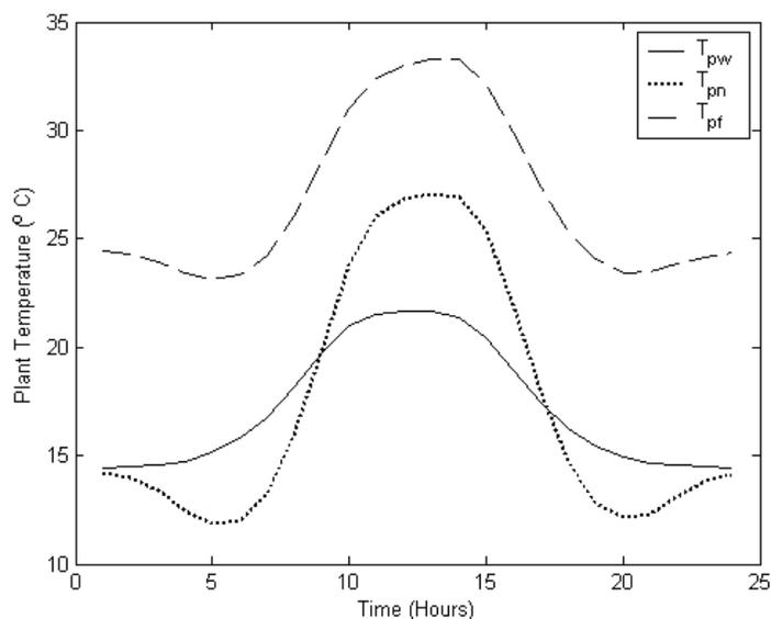
Figure 3(a). Hourly variation of plant temperature without north wall, with PCM north wall and with PCM floor.
