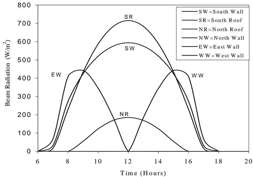
Figure 2 (a). Hourly variation of beam radiation on different walls and roofs of greenhouse for a typical winter day in New Delhi.
