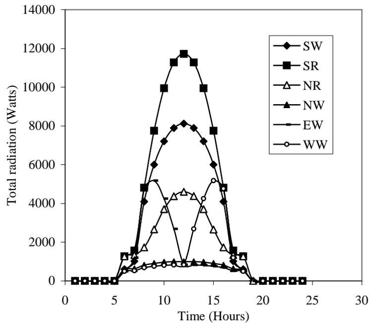
Figure 2 (b). Hourly variation of total solar radiation incident on greenhouse for a typical winter day in New Delhi.
