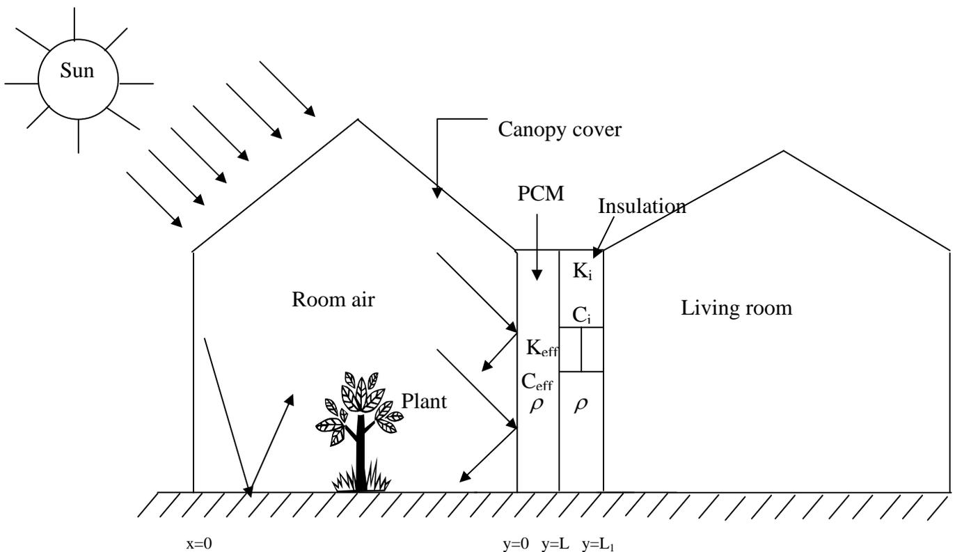
Figure 1(b). Schematic view of Greenhouse-cum-Solarium with insulated PCM north wall.
