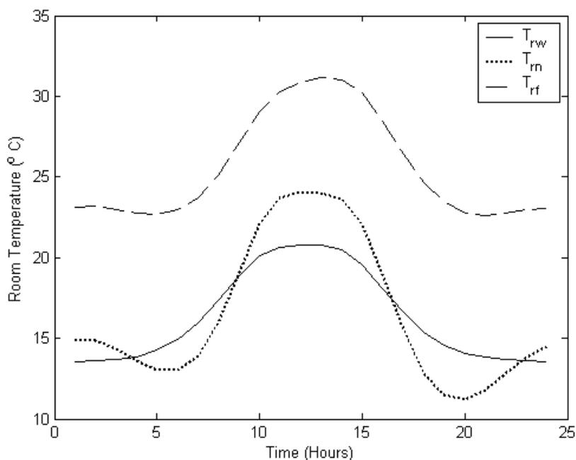
Figure 3(b). Hourly variation of room temperature without north wall, with PCM north wall and with PCM floor.
