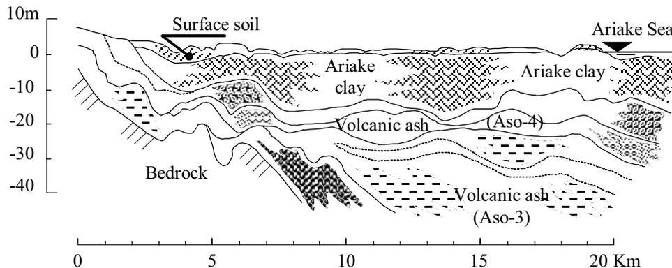
Figure 2. A typical geological profile.
