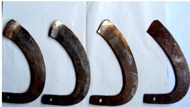
Figure 4 Blades with different tip angle
