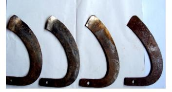
Figure 4 Blades with different tip angle
