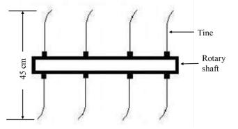
Figure 5 Blade arrangement of planter in ST mode
