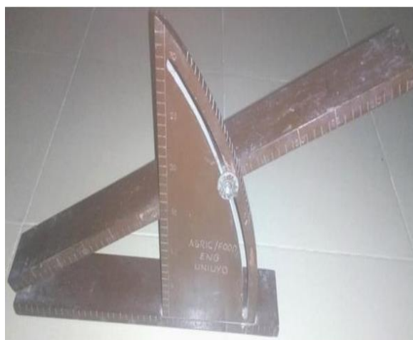
Figure 7 An inclined plane apparatus for determining coefficient of static friction
