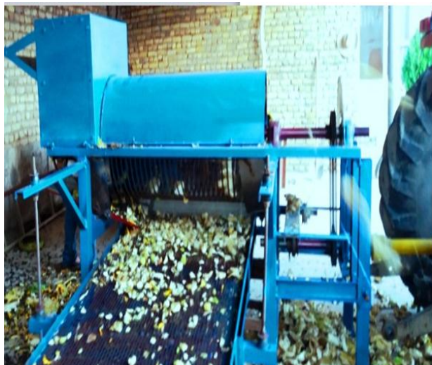
(1) input channel, (2) feeder, (3) beaters, (4) separator (concave), (5) thresher shaft, (6) covering of drum thresher, cleaner unit: (7) set of screens, (8) crank of oscillation (9) power transmission
