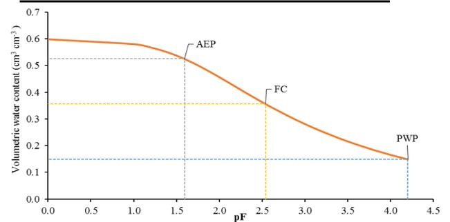
Figure 5 Water retention curve
